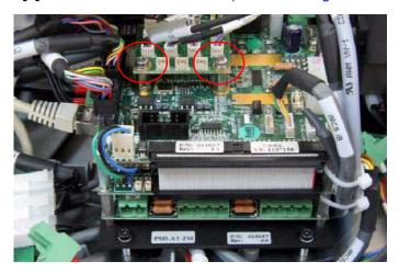
[3] Remove the 2 Phillips screws from the sensor board.
