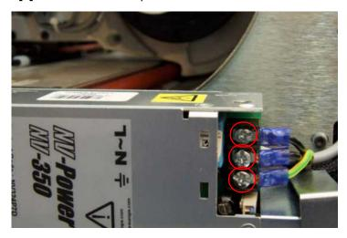
[6] Unscrew the 3 power cable lugs with a cross-head screwdriver.
