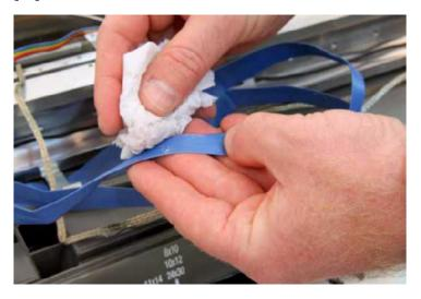
[12] Clean the ribbon cable to remove glue and other dirt.
