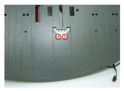
[5] Remove the 2 Phillips screws located on top of the tray.
