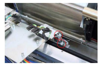
[6] Cut the 2 plastic cable ties on the right side of the laser board.
