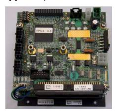
[7] Remove the four 2.5 mm Allen screws retaining the motion board and lift the board from the scanner.
