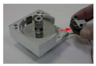
[9] Remove the encoder reader from the linear motor assembly.
