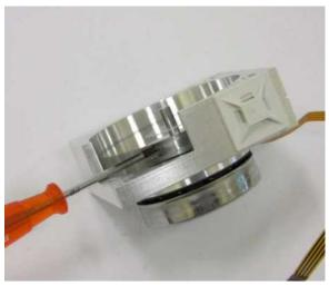
[12] Loosen the screw securing the encoder disc to the motor using the 0.89 Allen wrench.
