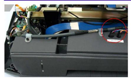
[3] Remove the solenoid cable plastic ties and disconnect the solenoid connectors.
