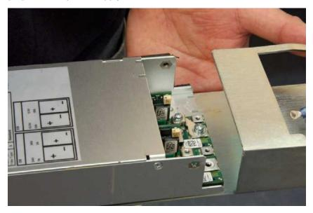
[17] Slide the power supply out of the power supply housing bracket.
