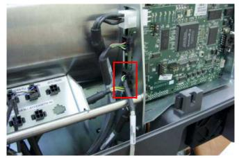
[1] Connect the barcode reader cable to J6 on the controller board.
