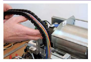
[15] Place the ribbon cables inside the U channel of the (female side) IGUS energy chain. The IGUS energy chain adjustment bracket is to the right.
