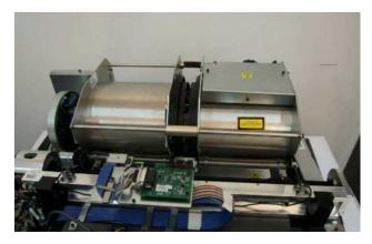
[3] Move the scanning head to the middle of the drum.
