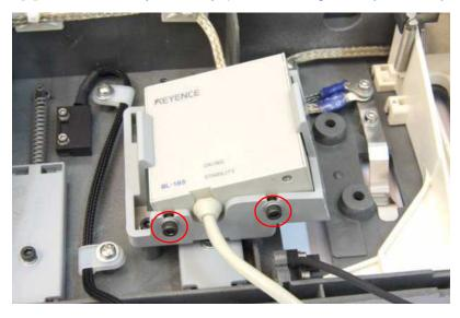
[4] Remove the barcode reader by opening the 4 Allen screws that attach the barcode reader to the old plastic housing.
