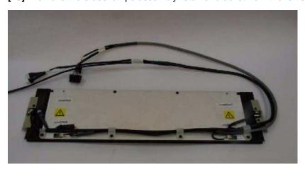
[11] Pull the erase lamps assembly out of the drum from the left side of the scanner.
