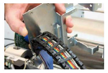
[16] Align the (male side) IGUS energy chain exactly over the female side (with the sensor board bracket to the left).
