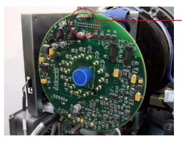
The ground connector is behind the board
